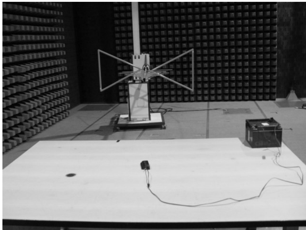
Photograph 2: Set-up for Radiation Measurement Below 1GHz
