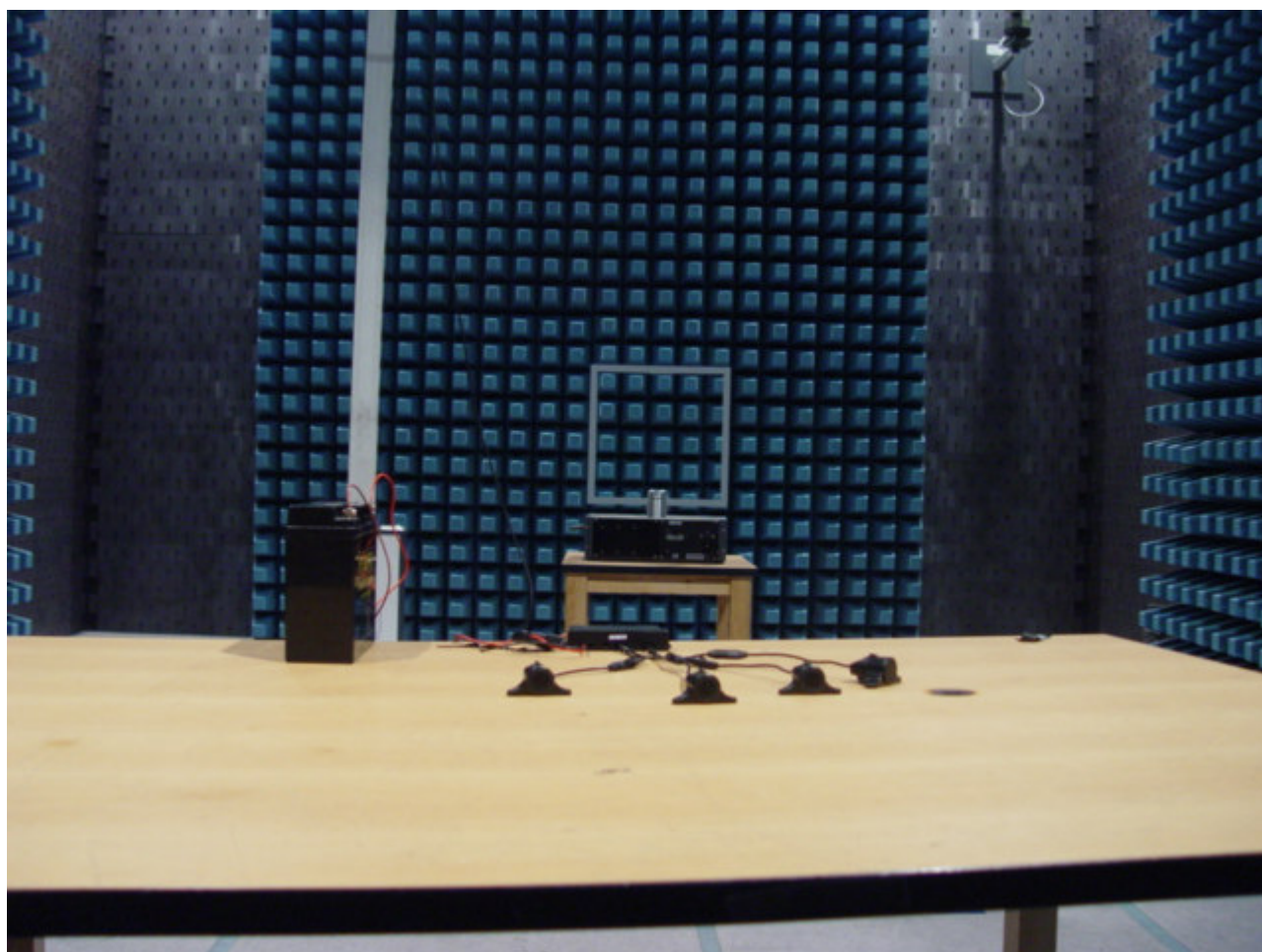
Photograph 1: Set-up for Radiation Measurement Below 30MHz
