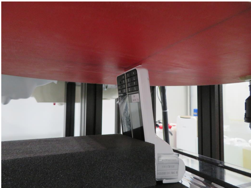
Description: Body Bottom with 0mm gap
