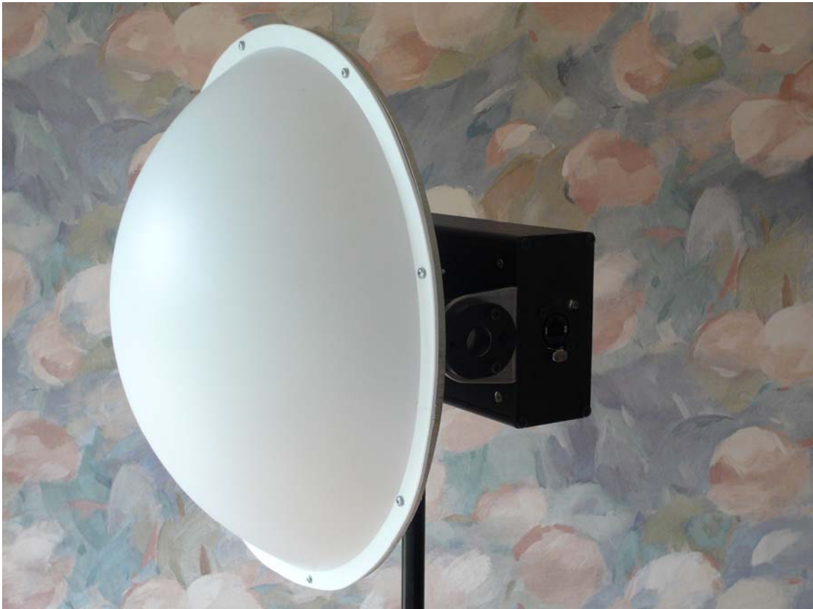
External view of Transmitter with parabolic antenna permanently attached
