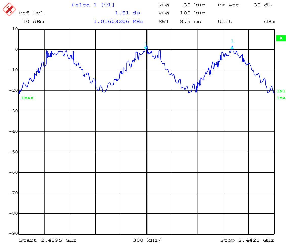
The hopping channel carrier frequencies are separated by a minimum of the 20 dB bandwidth of the hopping channel.
