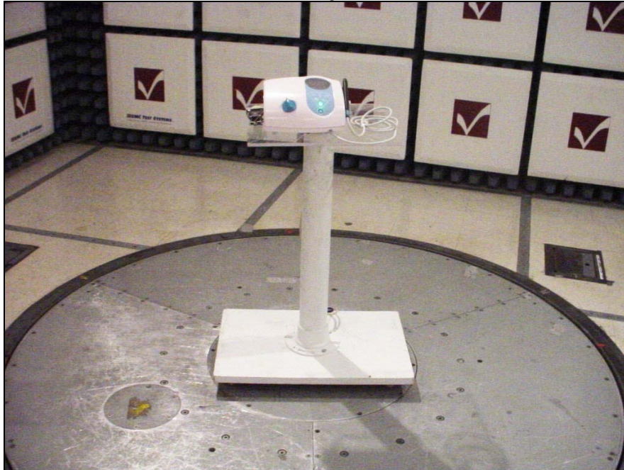
View of the EUT showing the setup on a pedestal during radiated emissions testing In stand-by mode.
