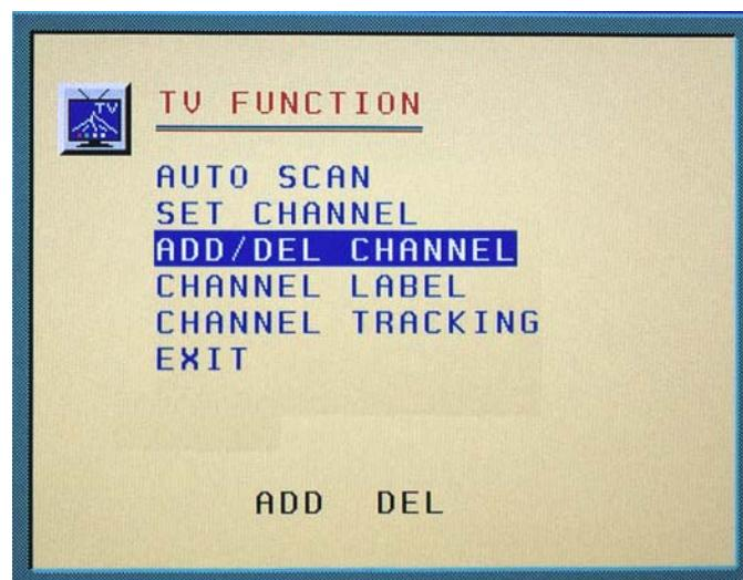
CHANNEL LABEL menu allows user to added TV preset channel with label.
