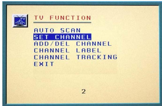
ADD / DEL CHANNEL menu allows user to add current channel to memory (store) or delete preset channel from memory (erase)
