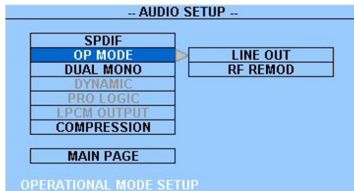
LINE OUT : Lineout mode, with digital dialog normalization.
