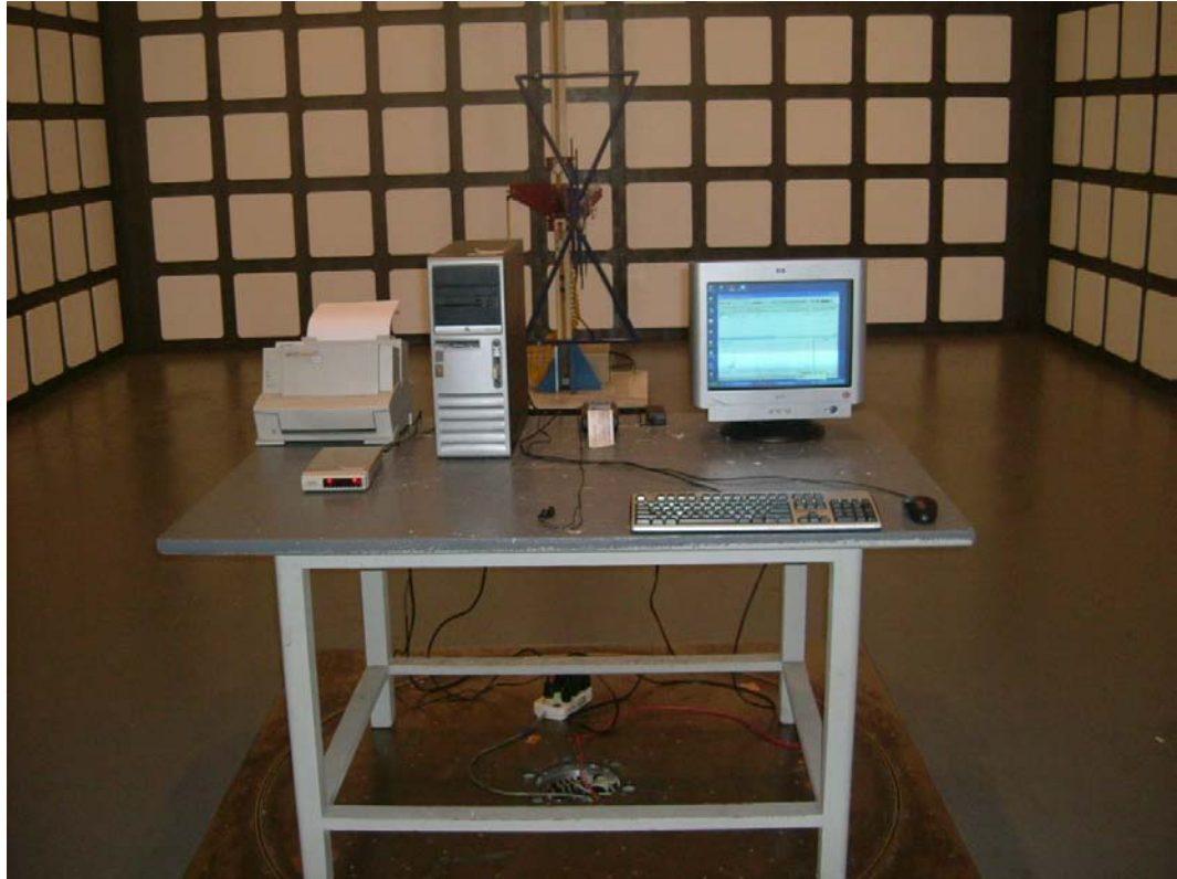
FRONT VIEW OF RADIATED EMISSION TEST (WITH MINI ADAPTOR)
