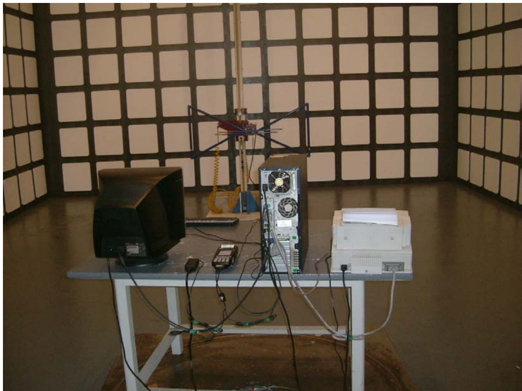
BACK VIEW OF RADIATED EMISSION TEST (WITH MINI ADAPTOR)
