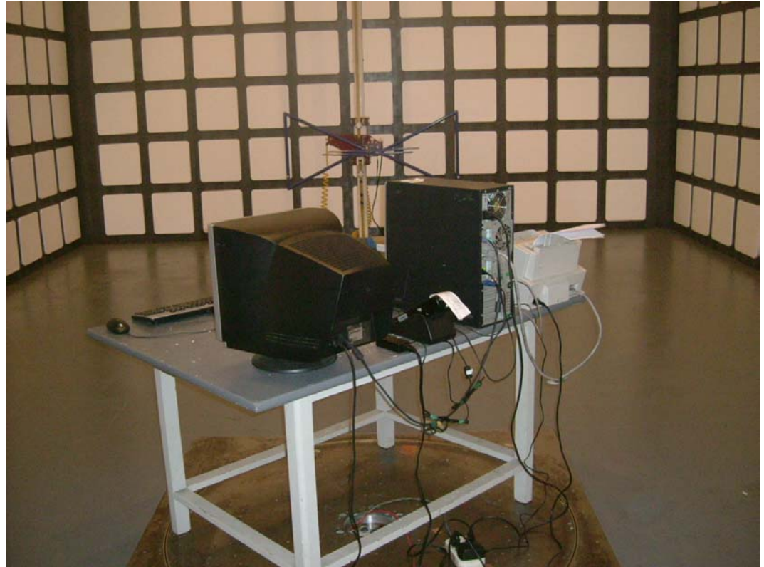
SETUP WITH MAXIMUM DETECTED EMISSION AT HORIZONTAL POLARIZATION (WITH CHARGER CRADLE)
