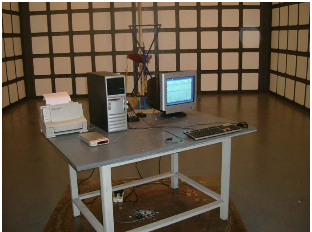
SETUP WITH MAXIMUM DETECTED EMISSION AT VERTICAL POLARIZATION (WITH CHARGER CRADLE)
