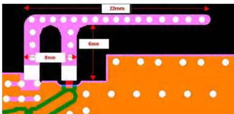
In this case the maximum dimension of the antenna is 17mm,  $\lambda_g/4$ . The antenna could also be 34 or 68mm long,  $\lambda_g/2$  and full  $\lambda_g$  respectively, depending on space available. The advantage of making it larger is greater bandwidth and immunity to de-tuning.
