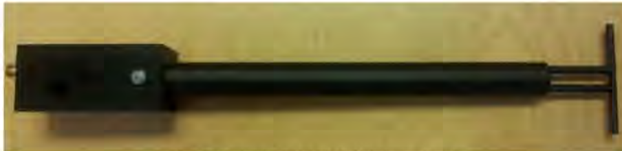
Figure 1 – MVG COMOSAR Validation Dipole
