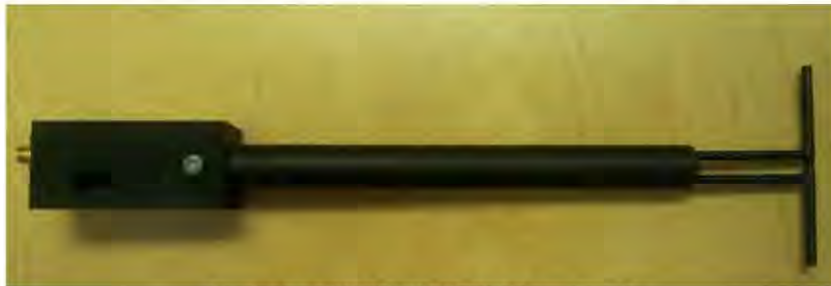
Figure 1 – MVG COMOSAR Validation Dipole
