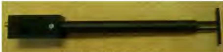
Figure 1 – MVG COMOSAR Validation Dipole
