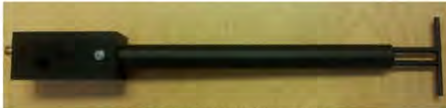
Figure 1 – MVG COMOSAR Validation Dipole
