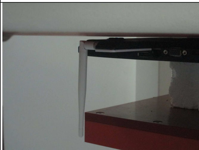
Test Position 4: USB Horizontal Down Dongle With 0.5 cm Gap (Antenna in Vertical 90 degree)
