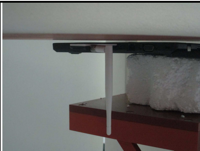
Test Position 2: USB Horizontal Up Dongle With 0.5 cm Gap (Antenna in Vertical 90 Degree)
