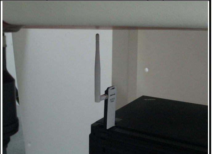
Test Position 12: USB Tip Mode Tip of Antenna with 0.5cm Gap (Antenna in Vertical 90 degree)
