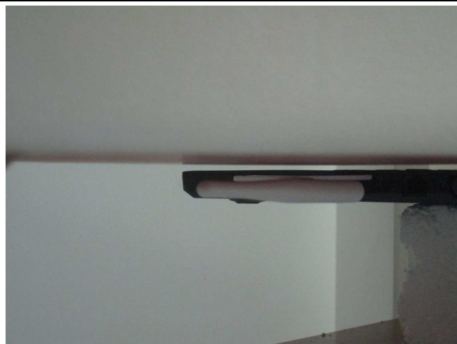
Test Position 1: USB Horizontal Up Both (Dongle and Antenna) With 0.5 cm Gap (Antenna in Vertical 180 degree)
