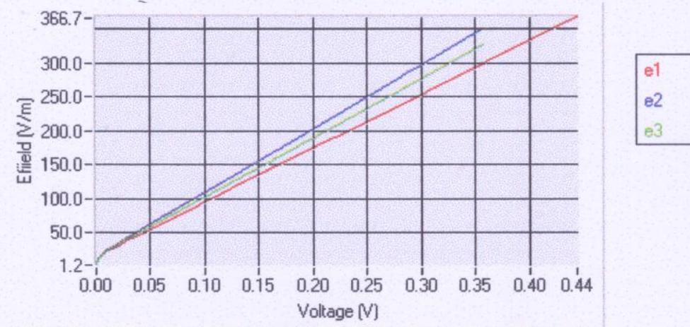
**Calibration coefficients for the three dipoles in CW:**
