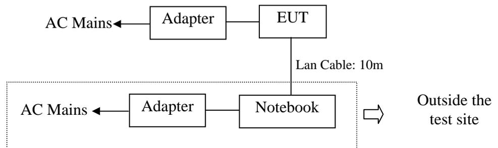
**(EUT: 150Mbps Wireless N ADSL2+ Modem Router)**
