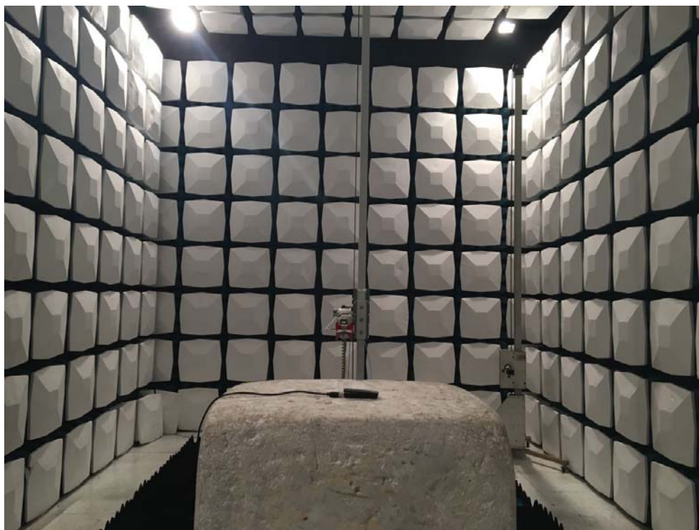
Description: Radiated Emission Test Setup for 1~18GHz
