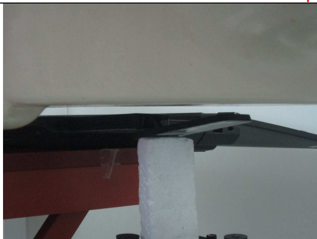
Test Position 6: USB Horizontal Up with 0.5 cm Gap (Antenna in open 175 degree)
