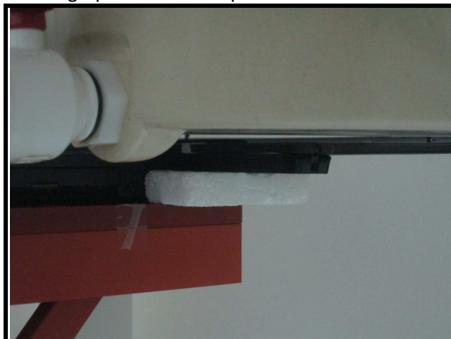
Test Position 1: USB Horizontal Up with 0.5 cm Gap
