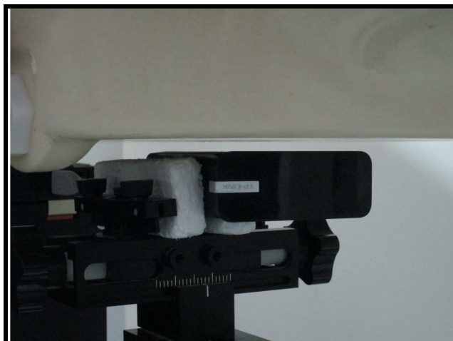
Test Position 13: USB Vertical Back with 0.5 cm Gap (Antenna in open 90 degree)
