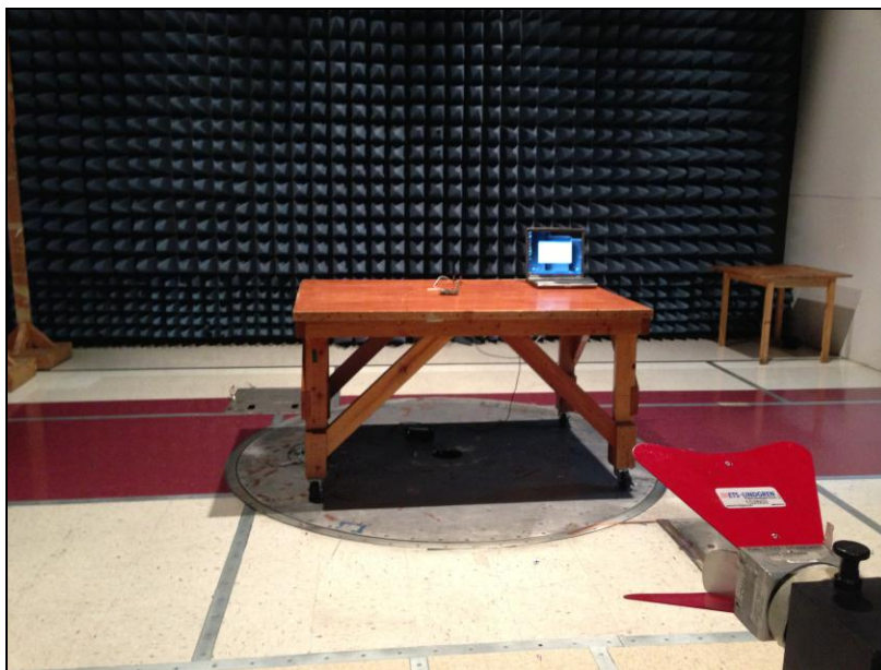
Photograph 12. Radiated Spurious Emissions, Test Setup above 1 GHz (3 Meter Distance for Radiated Band Edge)
