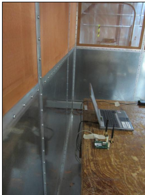
Photograph 8. Conducted Emissions, 15.207(a), Test Setup, Side View
