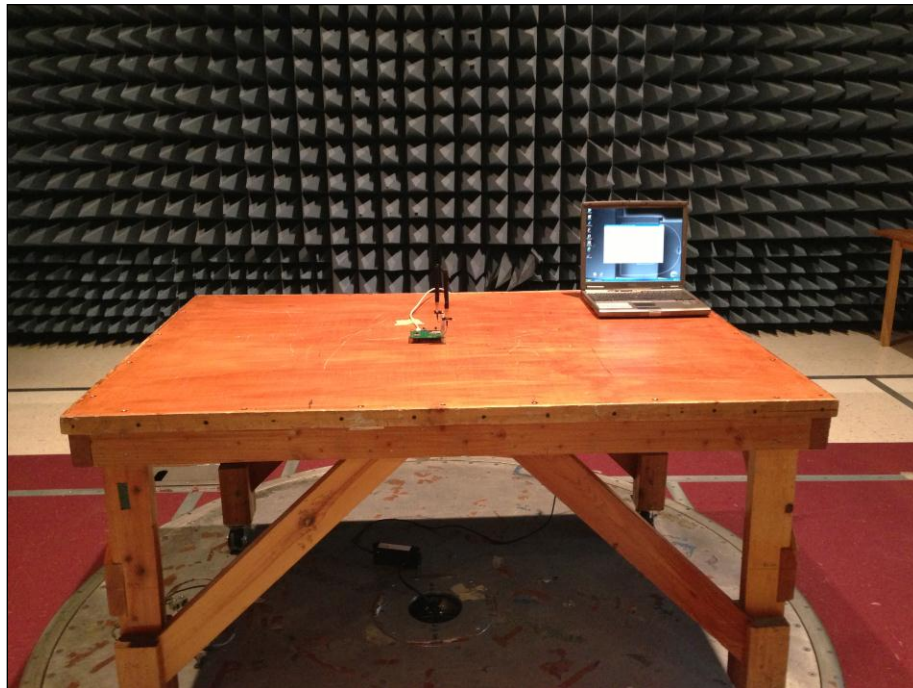
Photograph 8. Radiated Spurious Emissions, Test Setup
