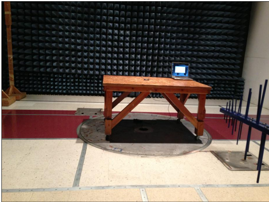
Photograph 4. Radiated Emissions, Test Setup, 30 MHz – 1 GHz
