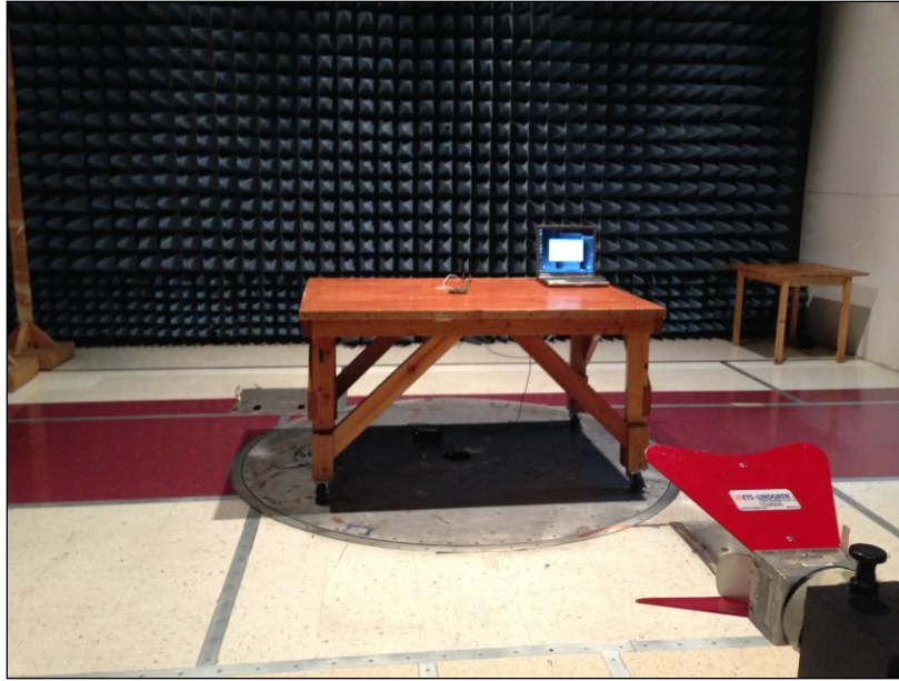
Photograph 11. Radiated Spurious Emissions, Test Setup above 1 GHz (3 Meter Distance for Radiated Band Edge)
