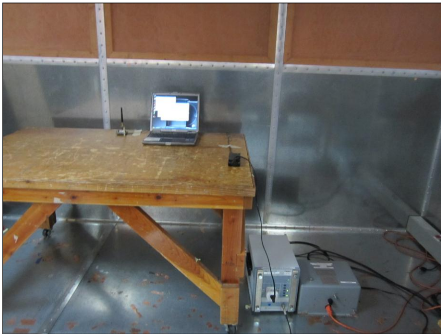
Photograph 6. Conducted Emissions, 15.207(a), Test Setup
