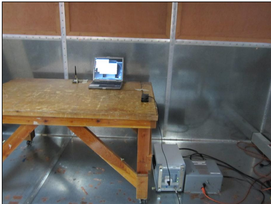
Photograph 7. Conducted Emissions, 15.207(a), Test Setup
