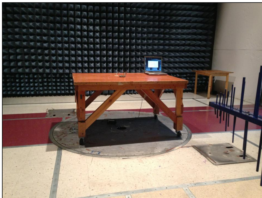
Photograph 10. Radiated Spurious Emissions, Test Setup 30MHz – 1GHz
