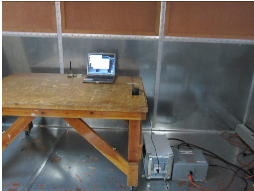
Photograph 2. Conducted Emissions, Test Setup
