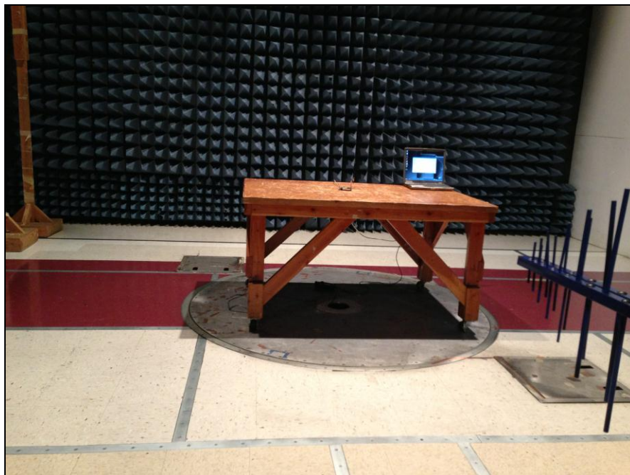
Photograph 5. Radiated Emissions, Test Setup, 30 MHz – 1 GHz
