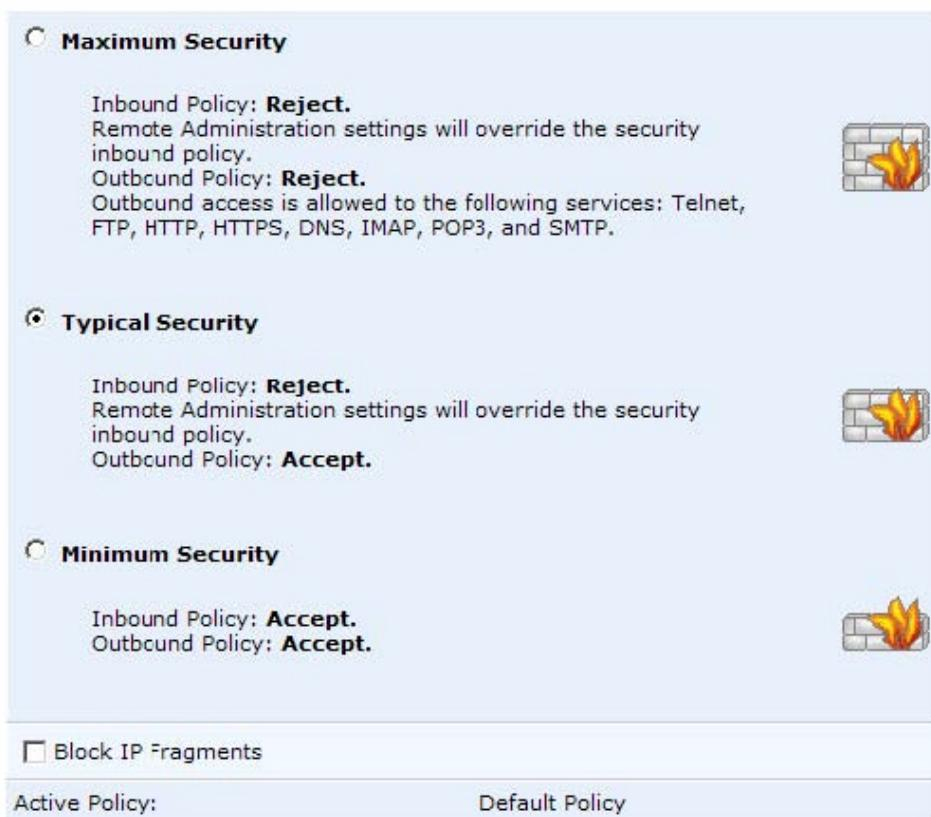
The Firewall regulates the flow of data between the enterprise network and the Internet. Both incoming and outgoing data are inspected and then accepted (allowed to pass through the CAP) or rejected (barred from passing through the CAP) according to a flexible and configurable set of rules. These rules are designed to prevent unwanted intrusions from the outside while allowing enterprise users access to the Internet services that they require.
