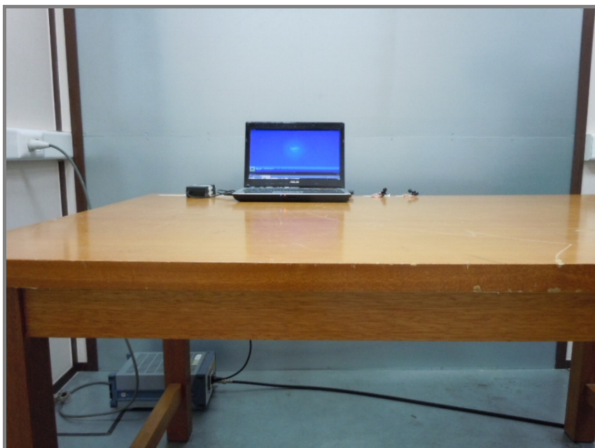
Photo of Conducted emission at below 30 MHz
