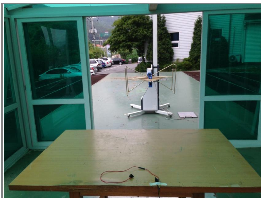
**Photo of radiated spurious emission at above 1 000 MHz**
