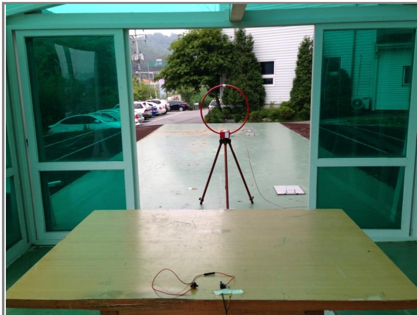
**Photo of radiated spurious emission at 30 MHz ~ 1 000 MHz**
