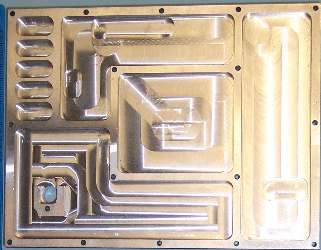
Note: PCB is bonded to the aluminum housing. There are no traces or components on the underside.
