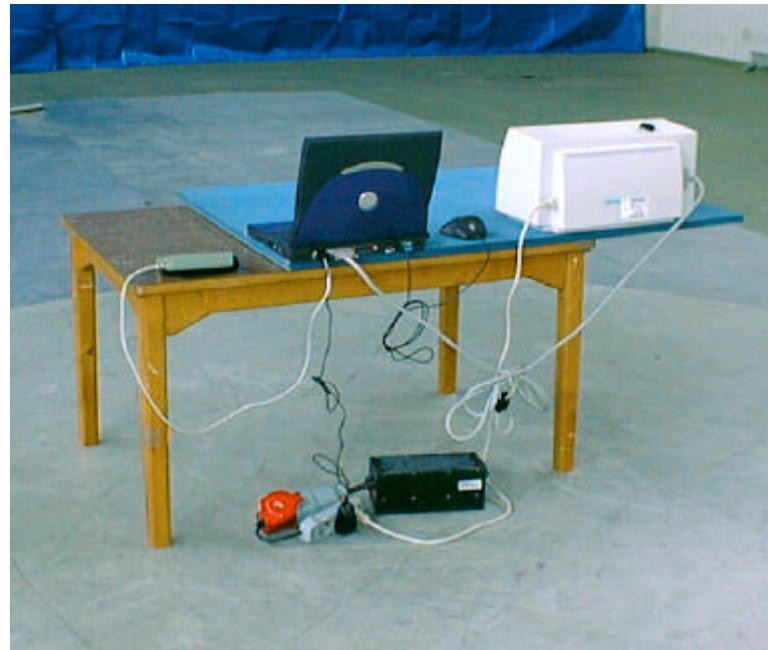
**Test set-up, Radiated Emission, receiver DBI 002**
