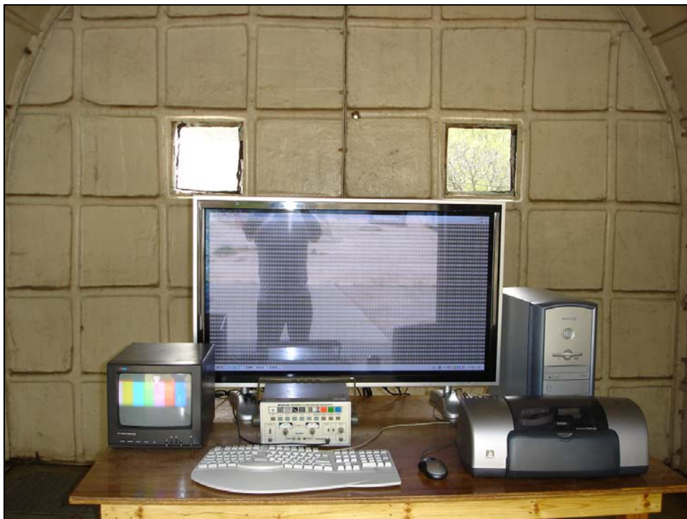
Photograph 2: Setup for Radiated Emissions
