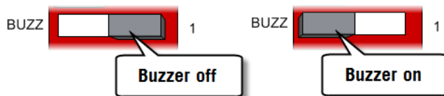
Figure 7.5. Setting the channel monitor buzzer with front-panel dip switch 1
