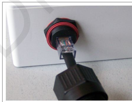
Figure 6.15. Connect cable to input jack
