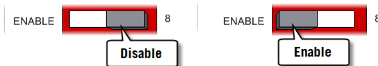
Figure 7.2. Enabling (disabling) a channel with front-panel dip switch 8
