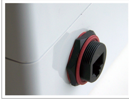
Figure 6.7. Inspect the factory-installed gasket
