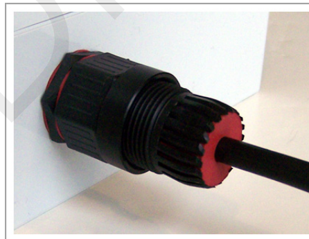
Figure 6.18. Proper fit of cable bushing into connector B
