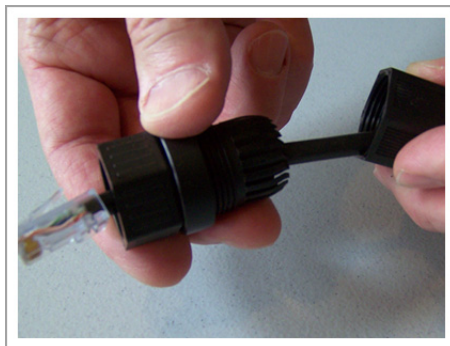
Figure 6.10. Thread cable through connector B
