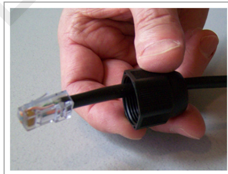
Figure 6.9. Thread cable through connector A
