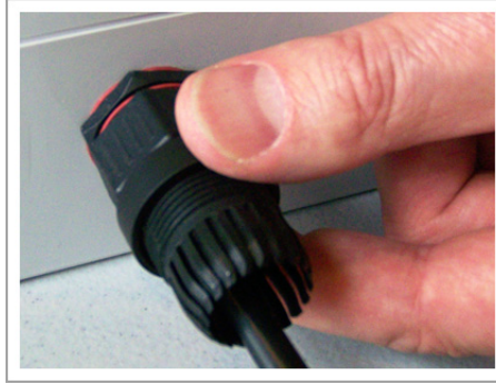
Figure 6.16. Thread connector B onto the SPP and hand tighten
