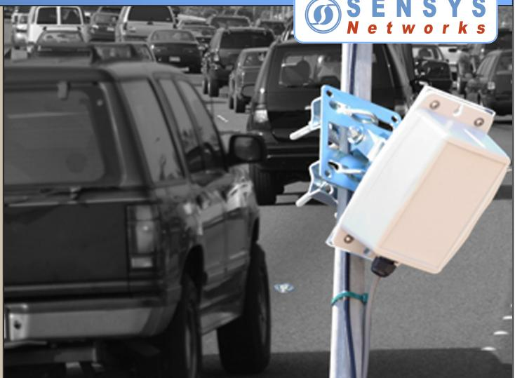
The Sensys Networks AP240-E is the high-end access point for the VDS240 family of wireless sensor vehicle detection products. It offers a rich set of features that simplify installation, traffic monitoring, and data reporting. The AP240-E contains both a host processor and a number of communications interfaces, including a radio transceiver to the VSN240 in-pavement wireless sensors, an Ethernet port, 2 serial ports, and options for GPRS/CDMA and GPS radios.
