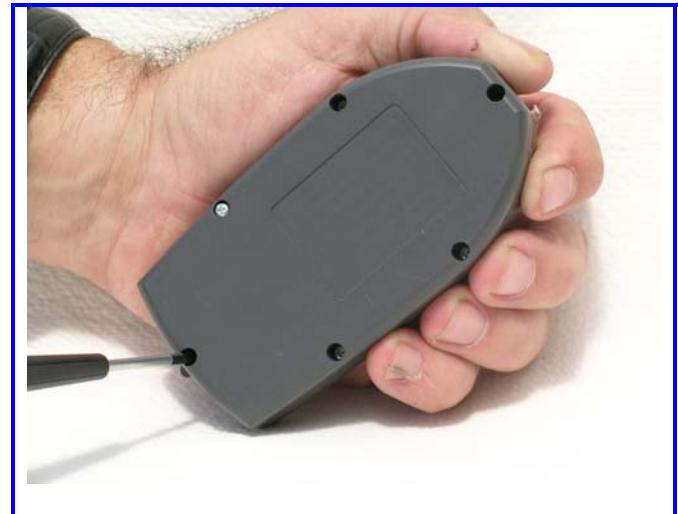
To access the battery, remove the six screws that keep the lower and top cover together
