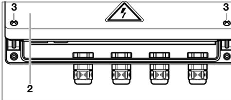
Remove the maintenance cover plate **2** on the voltage-free EXAConnect by unscrewing the two small bottom Phillips screws **3**. You thus gain access to the backup battery **37**.
