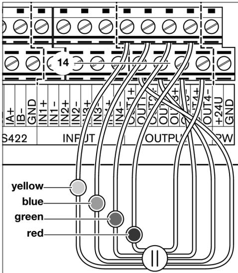
Pass the cable of the signal lamp through the opening of the cable entrance slot **8** to the 24 V output **14** on the terminal strip. The 24 V output is constructed with optocouplers for potential-free output of 24 V signals. Up to 3 A may be connected.
