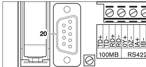
The baud rate of the RS232 interface is fixed at 9600 baud, 8 data bits, no parity, 1 stop bit (8N1). The RS232 interface uses no handshake at all. It is constructed as DCE (data communication equipment) and is non-potential-free.
