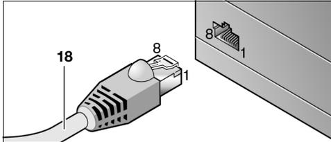
For a 1:1 connection, insert the plug into a free network outlet of your firm network.
