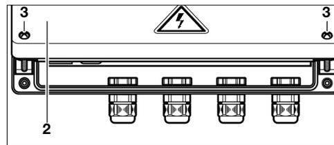
Remove the maintenance cover plate **2** on the voltage-free EXAConnect by unscrewing the two small bottom Phillips screws **3**. You thus gain access to the reset button **39**.
