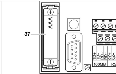
Remove the old battery **37** and insert a new standard AAA microcell battery.
