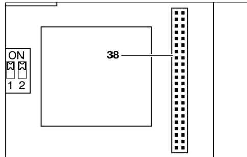
The bus slot **38** offers the possibility of connecting additional hardware cards (e.g., a graphics card). Such cards are available as accessories.
