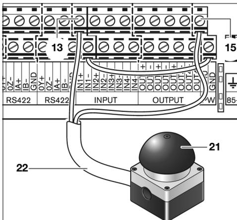
In the EXACConnect, connect one lead of the “GND” terminal of the direct current output **15** to the matching “IN-” terminal of the 24 V input **13**. When, for example, you have connected one lead of the cable **22** of the release button to the “IN1+” terminal of the 24 V input **13**, you must then connect the internal lead to the “IN1-” terminal.
