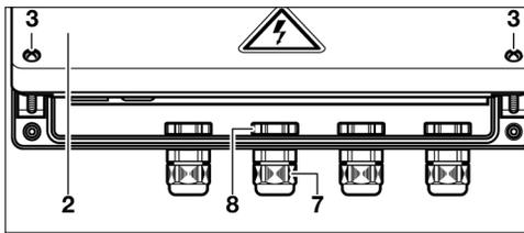
Remove the maintenance cover plate **2** on the voltage-free EXACConnect by unscrewing the two small bottom Phillips screws **3**. You thereby gain access to the terminal strip **9**.
