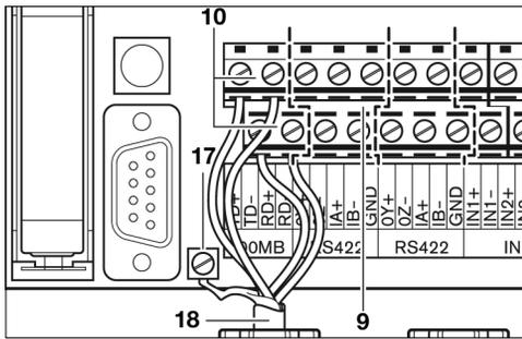
Cut off one plug on the twisted pair cable **18** for Ethernet networks. Pull the cable through the opening of the left cable entrance slot **8** to the terminal strip **9**.
