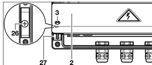
For wall mounting of the EXAConnect, you will need two M4 screws **26** having a head diameter of 8 mm and a length of 20 mm. Insert the screws into the recess **27** on the left and right edge of the EXAConnect and screw it tightly to the wall.
