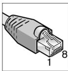
On the remaining plug of the twisted pair cable, determine which color lies on which pin. Use the following table to determine which leads you need for the connection to the EXAConnect and insulate the leads that are not needed. Connect the remaining leads to the Ethernet connection **10** of the terminal strip **9** in accordance with the table. Connect the shielding of the twisted pair cable to the grounding terminal **17**.
