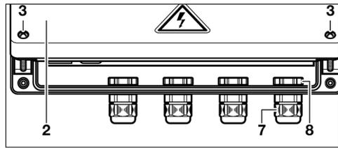
Remove the maintenance cover plate **2** on the voltage-free EXAConnect by unscrewing the two small bottom Phillips screws **3**. You thereby gain access to the terminal strip **9**.
