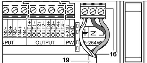
Connect the phase lead (brown wire) to the symbol  $\text{Ⓛ}$ , the neutral lead (blue wire) to the symbol  $\text{Ⓝ}$ , and the grounding lead (green-yellow striped wire) to the symbol  $\text{Ⓧ}$  of the mains connection **16**. **Always take care that the EXAConnect is grounded!**
