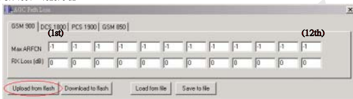
Figure 13 Click [Upload from flash] button to read value from flash
