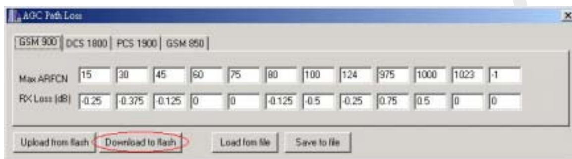
Figure 16 Click [Download to flash] button to write value to flash
