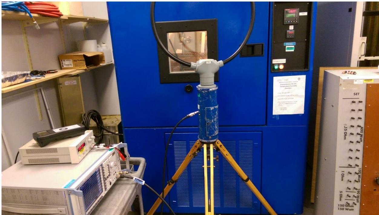
**Frequency Stability Test Setup**
