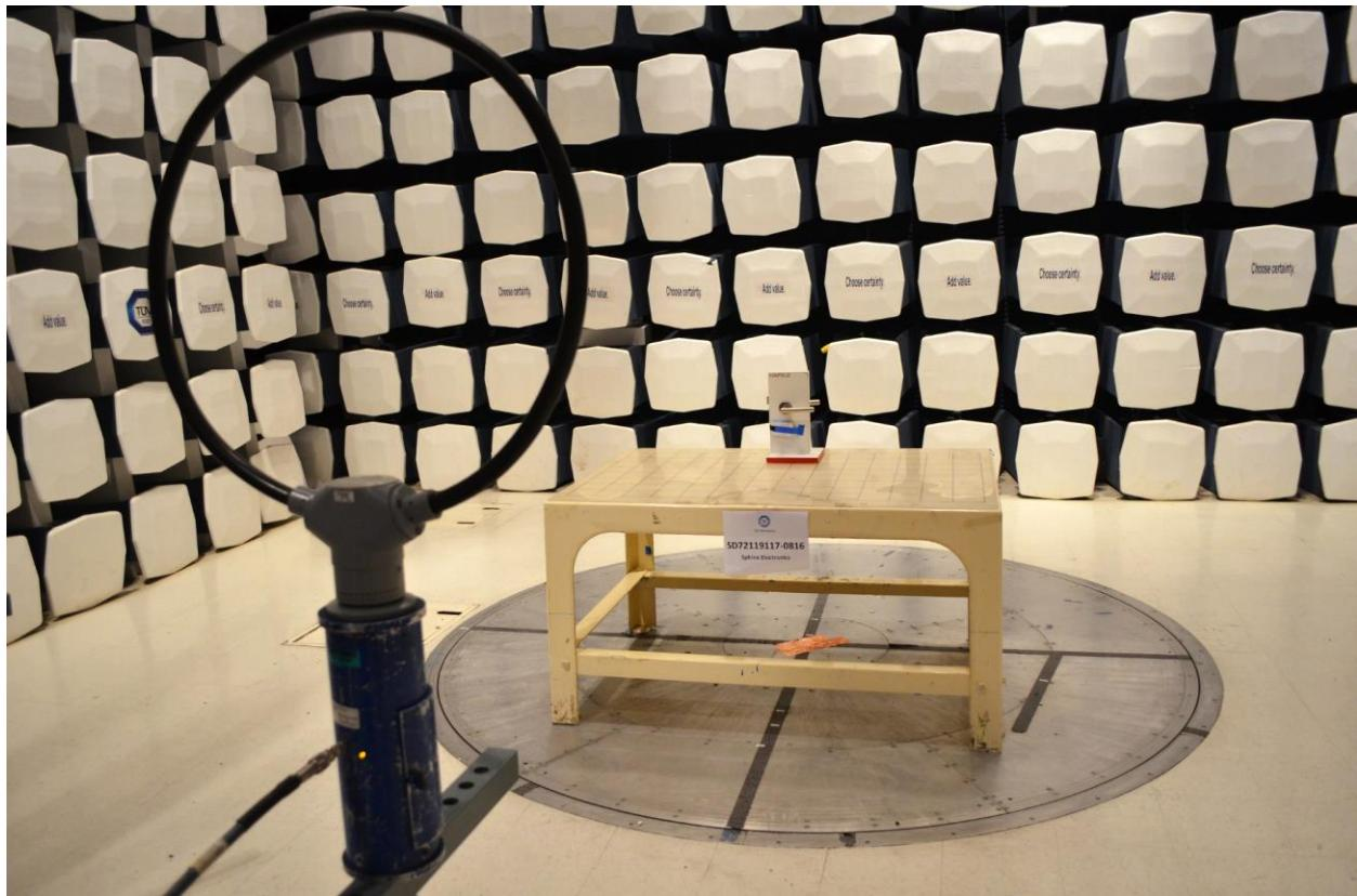
**Radiated Emissions Test Setup (below 30 MHz Front)**
