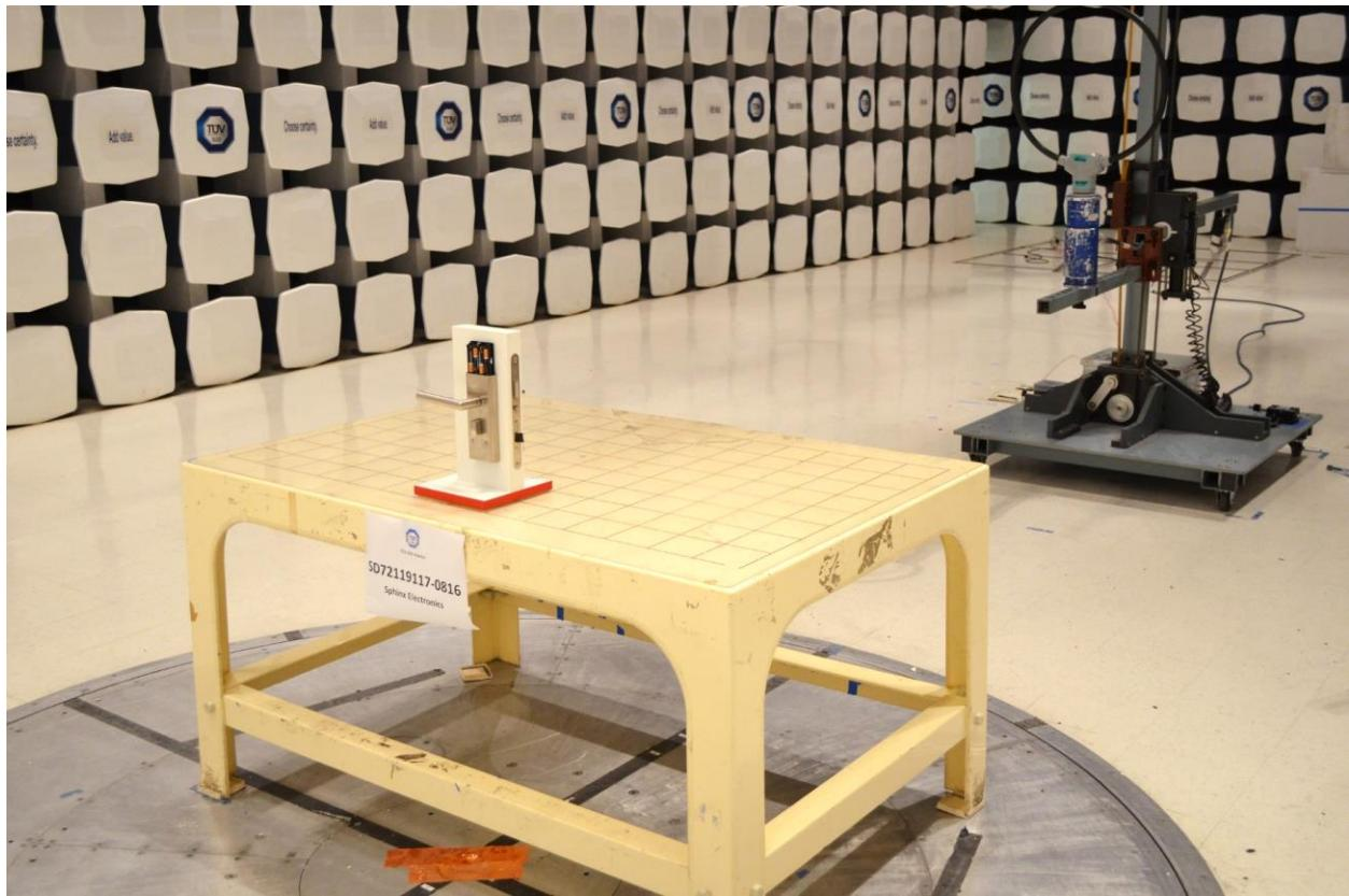
**Radiated Emissions Test Setup (below 30 MHz Back)**
