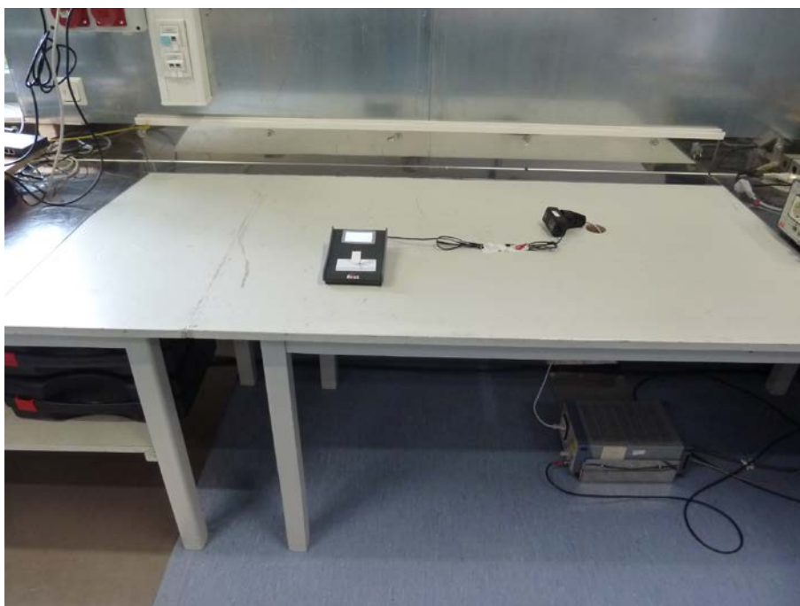
Photo 6: Test setup for conducted emissions
