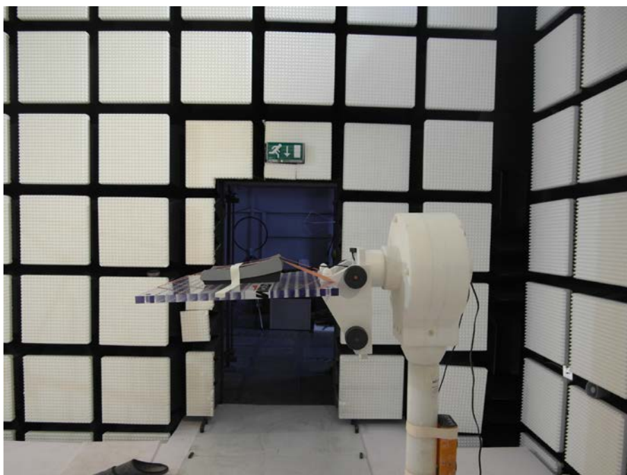
Photo 2: Test setup for radiated 9 kHz to 30 MHz
