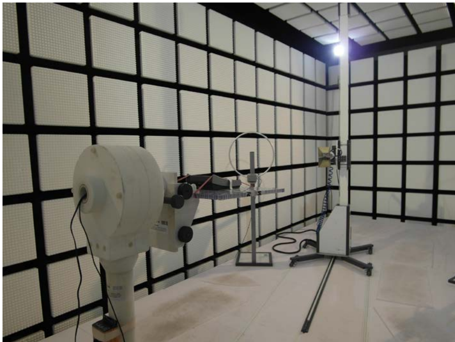
Photo 3: Test setup for radiated 9 kHz to 30 MHz
