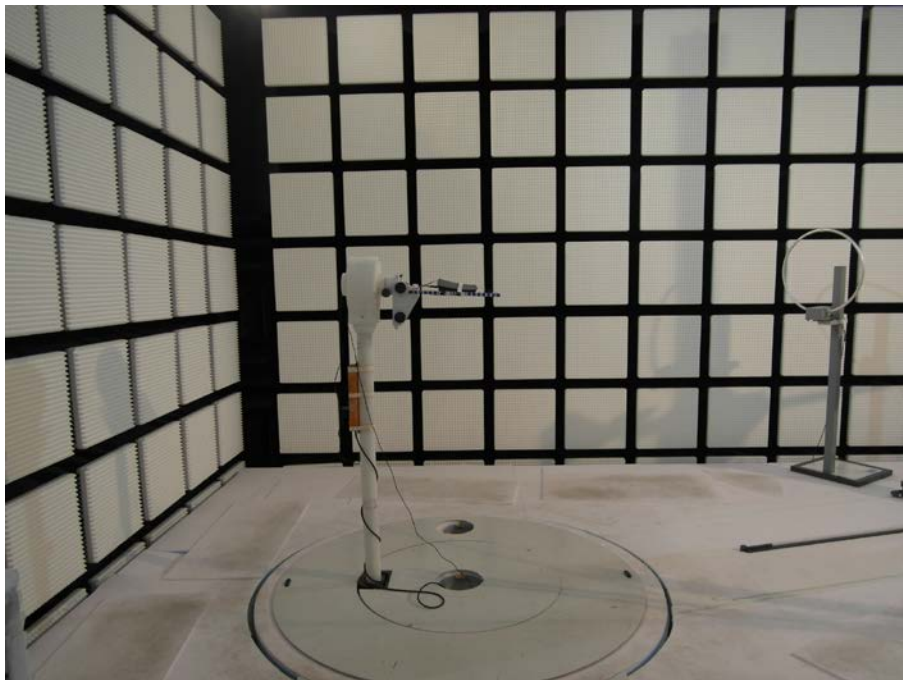
Photo 1: Test setup for radiated 9 kHz to 30 MHz
