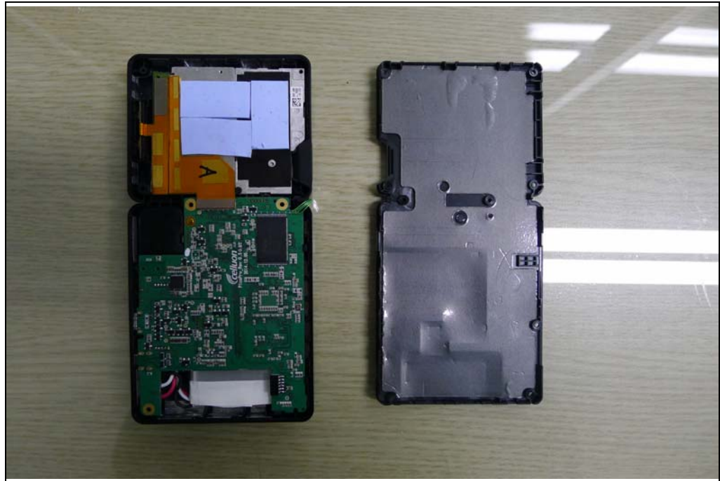
WLAN Module – Internal PCB Antenna
