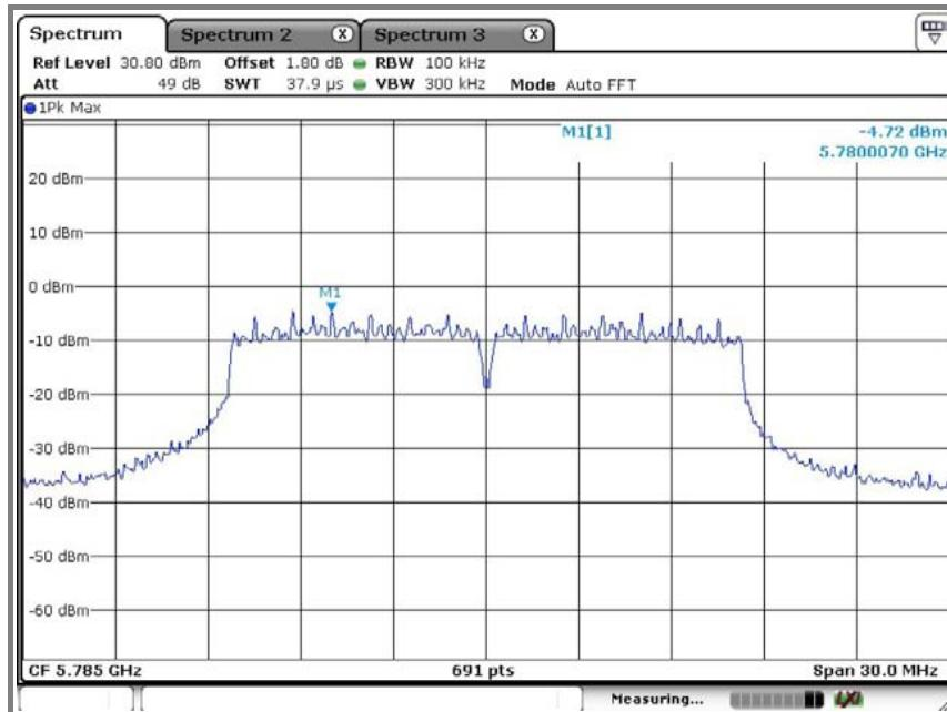
**Emission level measurement 1**
