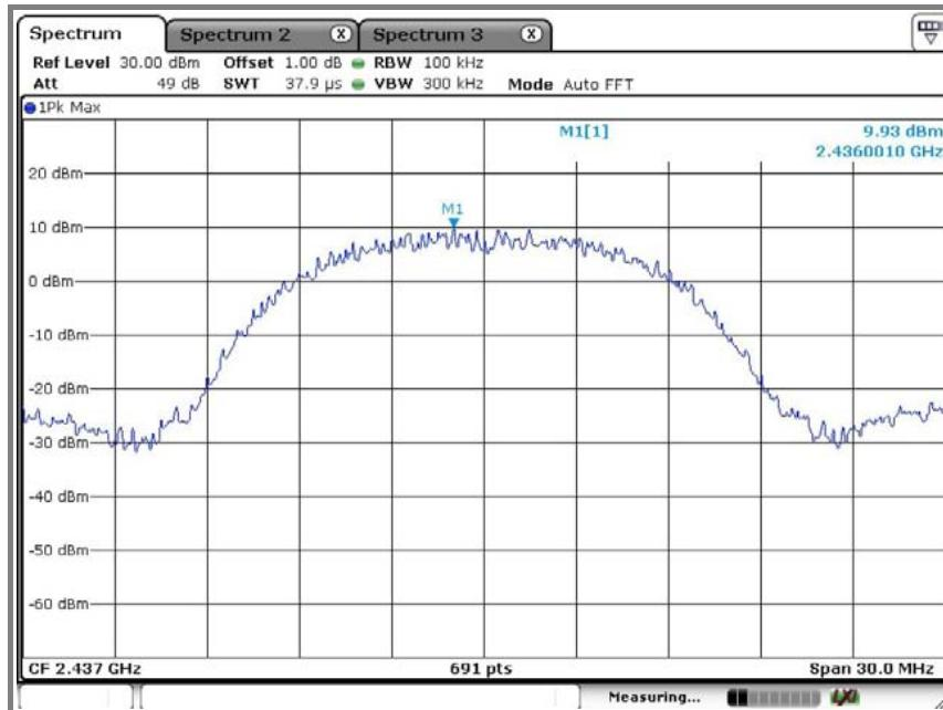
**Emission level measurement 1**
