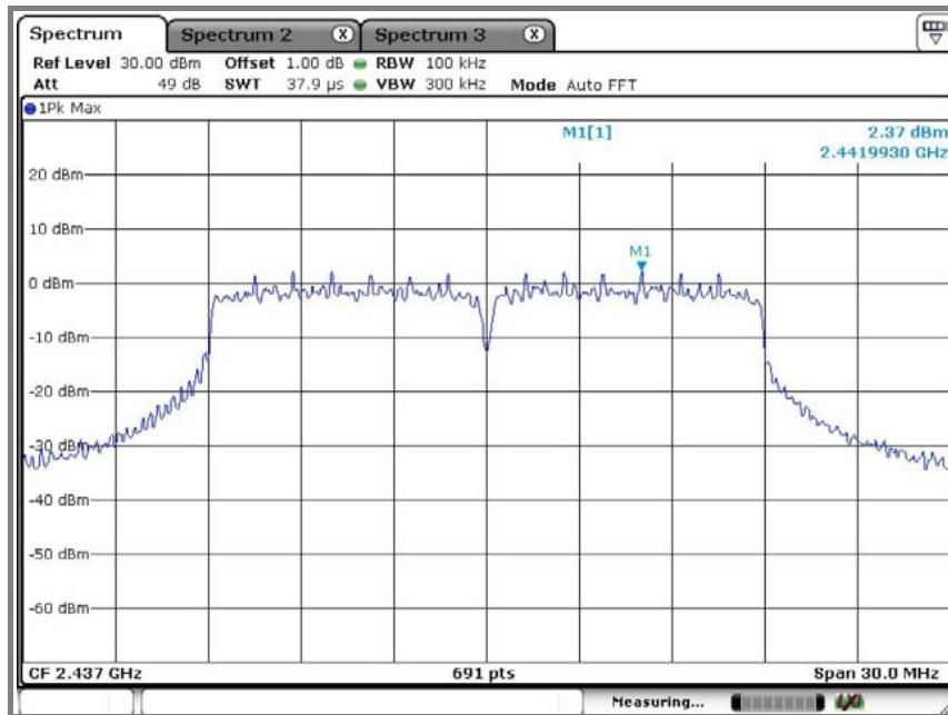
**Emission level measurement 1**
