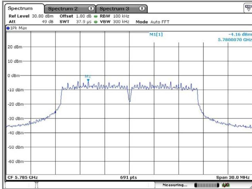
**Emission level measurement 1**
