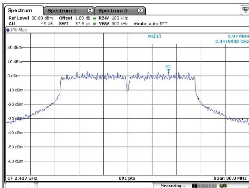
**Emission level measurement 1**
