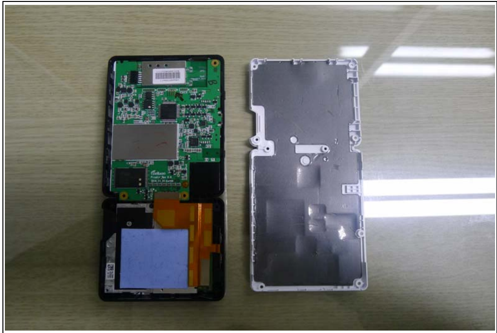
WLAN Module – Internal PCB Antenna
