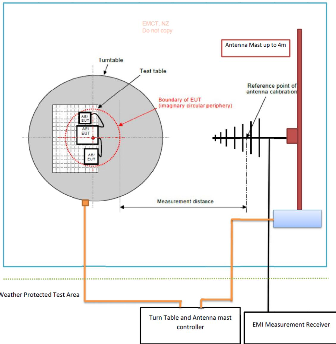
30 MHz-300 MHz: Bi conical Antenna; Measurement distance: 3 m
