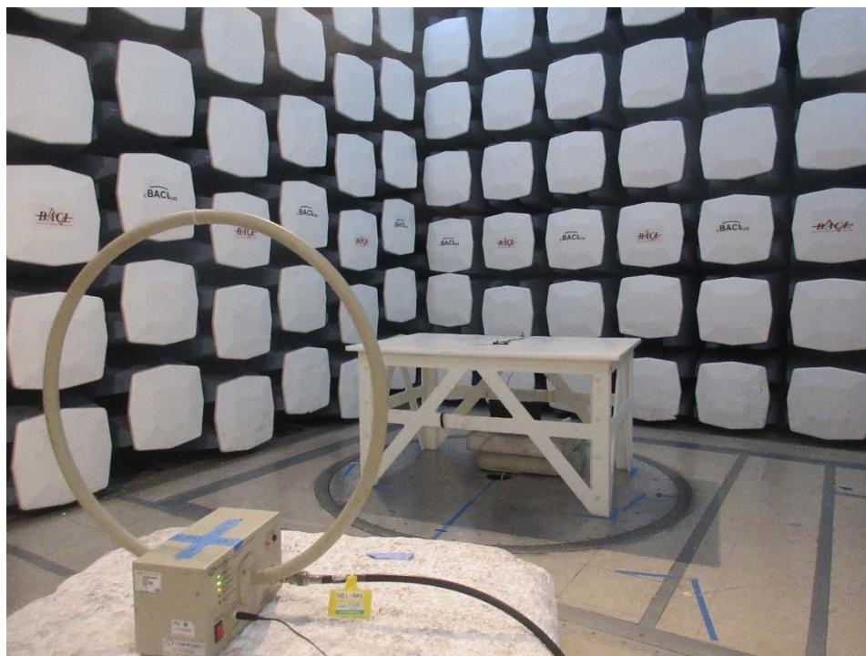
**1.4 Radiated Spurious Emissions: 9 kHz – 30 MHz, Perpendicular Rear View at 3 meters**
