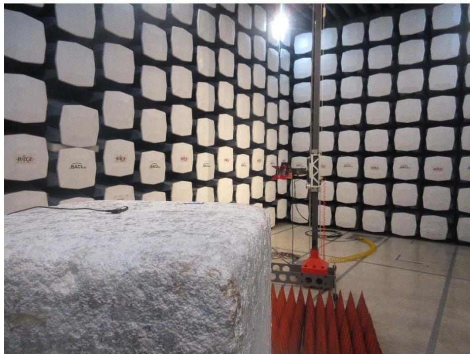
**1.9 Radiated Spurious Emissions: 18-26.5 GHz Front View at 3 meter**
