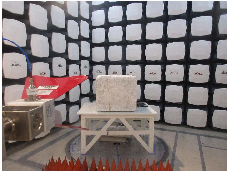
**1.8 Radiated Spurious Emissions: 1-18 GHz Rear View at 3 meter**
