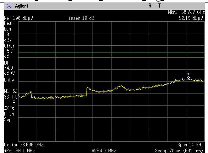
IC_U-NII-1_5200MHz_low_Mid Ch_40_20MHz BW_n-mode_15.209_26-49GHz_Peak_Port 2
