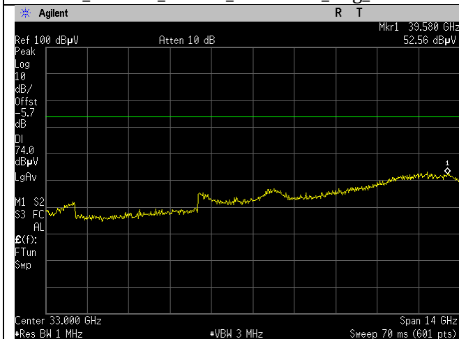
IC_U-NII-1_5200MHz_low_Mid Ch_40_20MHz BW_n-mode_15.209_26-49GHz_Peak_Port 1
