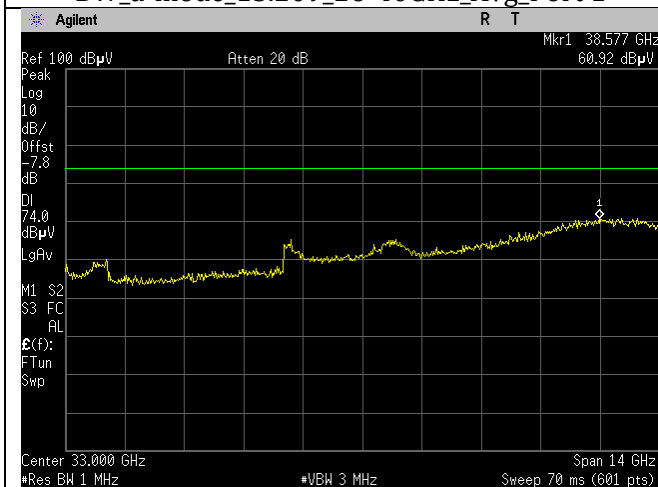
IC_U-NII-1_5200MHz_low_Mid Ch_40_20MHz BW_a-mode_15.209_26-49GHz_Peak_Port 1
