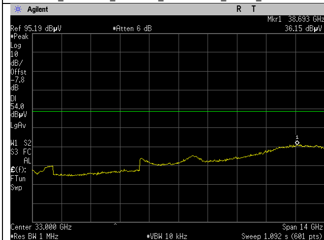
IC_U-NII-1_5200MHz_low_Mid Ch_40_20MHz BW_a-mode_15.209_26-40GHz_Avg_Port 1
