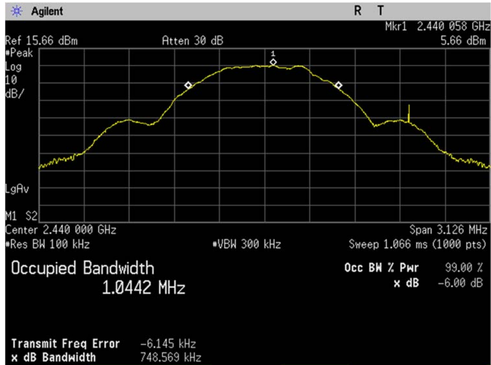
BLE_Mid Ch_2440MHz_1MBit_Occupied Bandwidth_-6dB_Port 1
