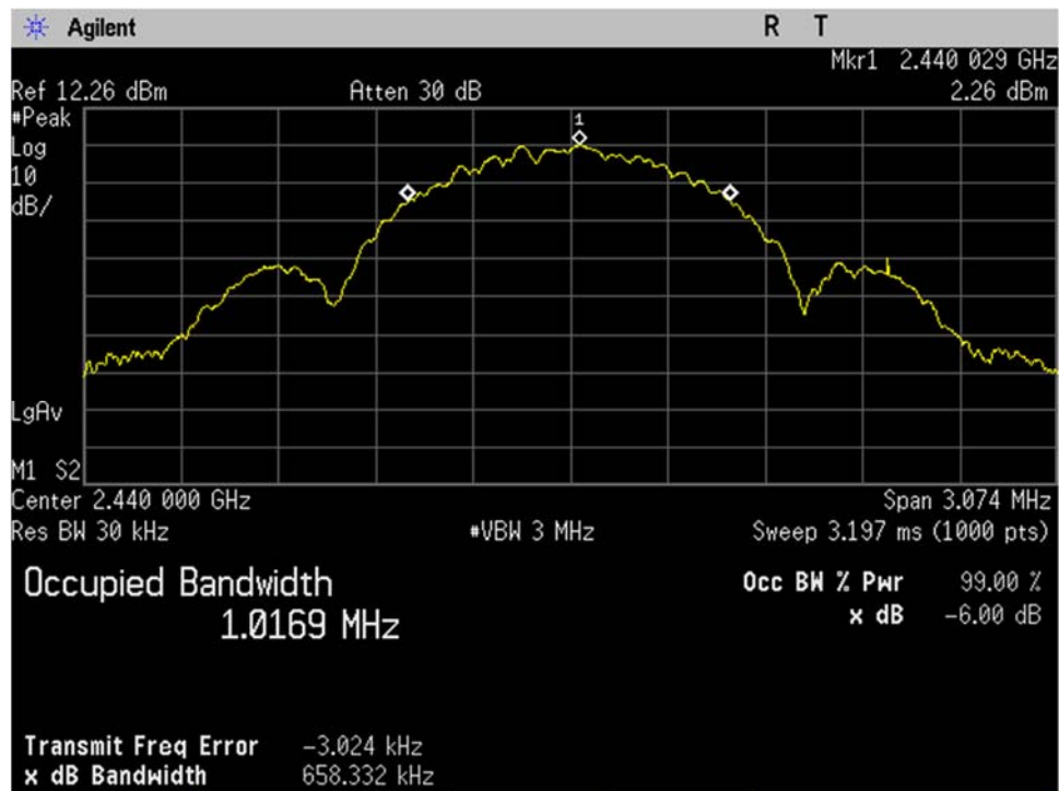
BLE_Mid Ch_2440MHz_1MBit_Occupied Bandwidth_99 percent_Port 1
