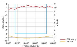
• Tested antenna has been soldered. Evaluation board size is 50x20x1 mm.
