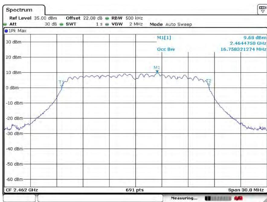
**802.11n20 mode****Low Channel 6 dB OBW Antenna A**
