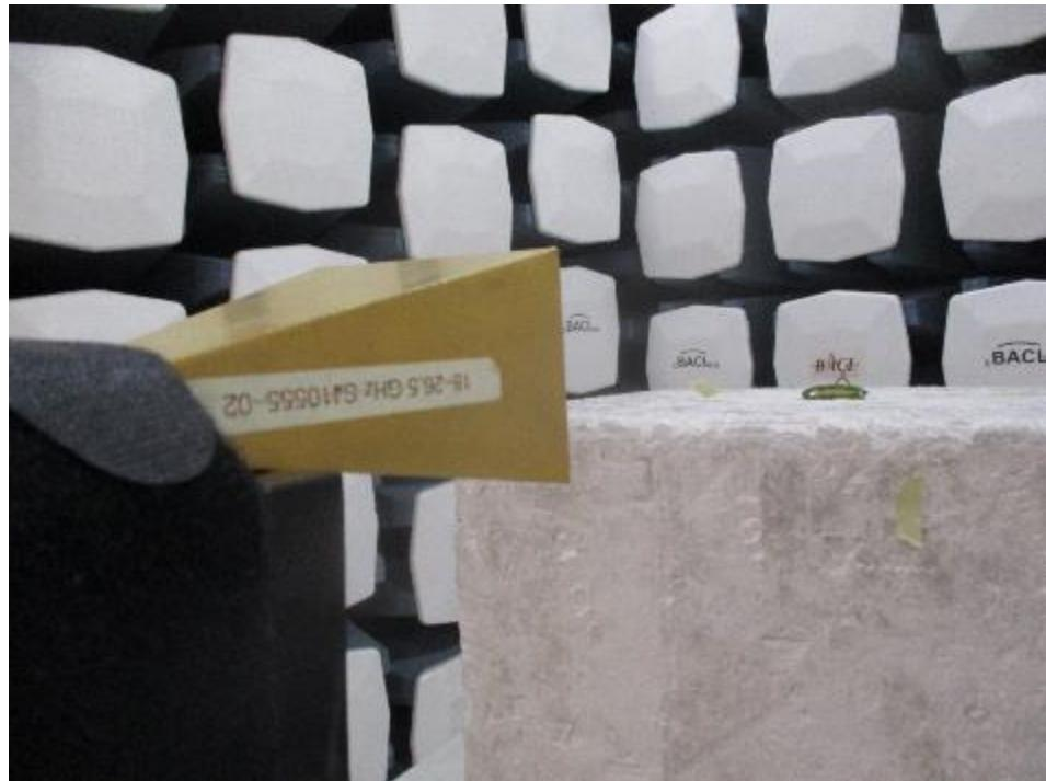
**1.6 Radiated Spurious Emissions: 18-26.5 GHz Rear View at 1 meter**
