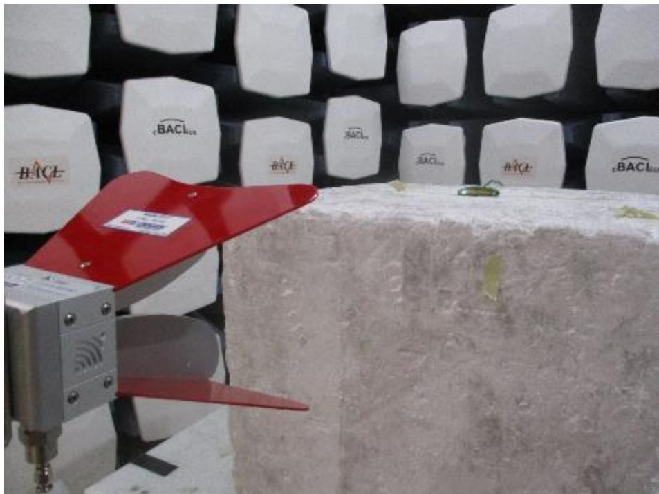
**1.4 Radiated Spurious Emissions: 1-18 GHz Rear View at 1 meter**
