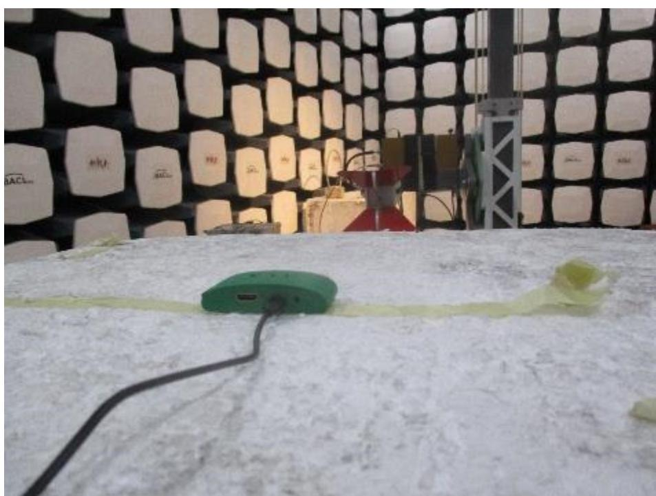
**1.5 Radiated Spurious Emissions: 18-26.5 GHz Front View at 1 meter**
