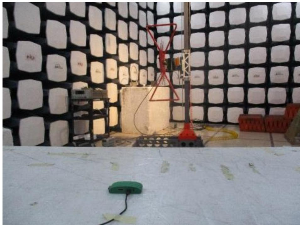
**1.3 Radiated Spurious Emissions: 1-18 GHz Front View at 1 meter**
