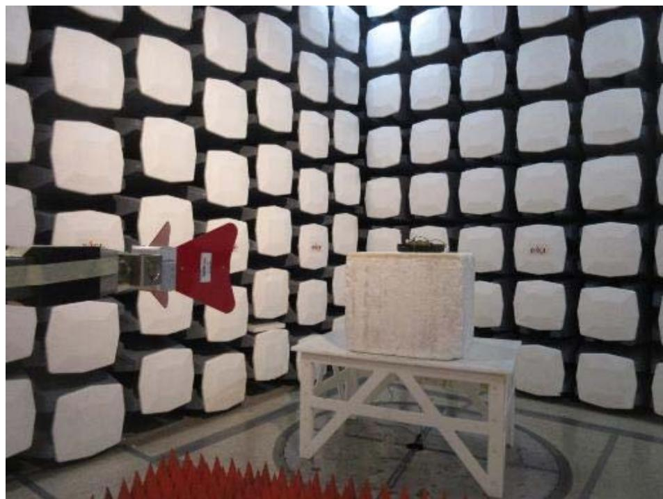
**1.4 Radiated Spurious Emissions: 1-18 GHz Rear View at 3 meters**
