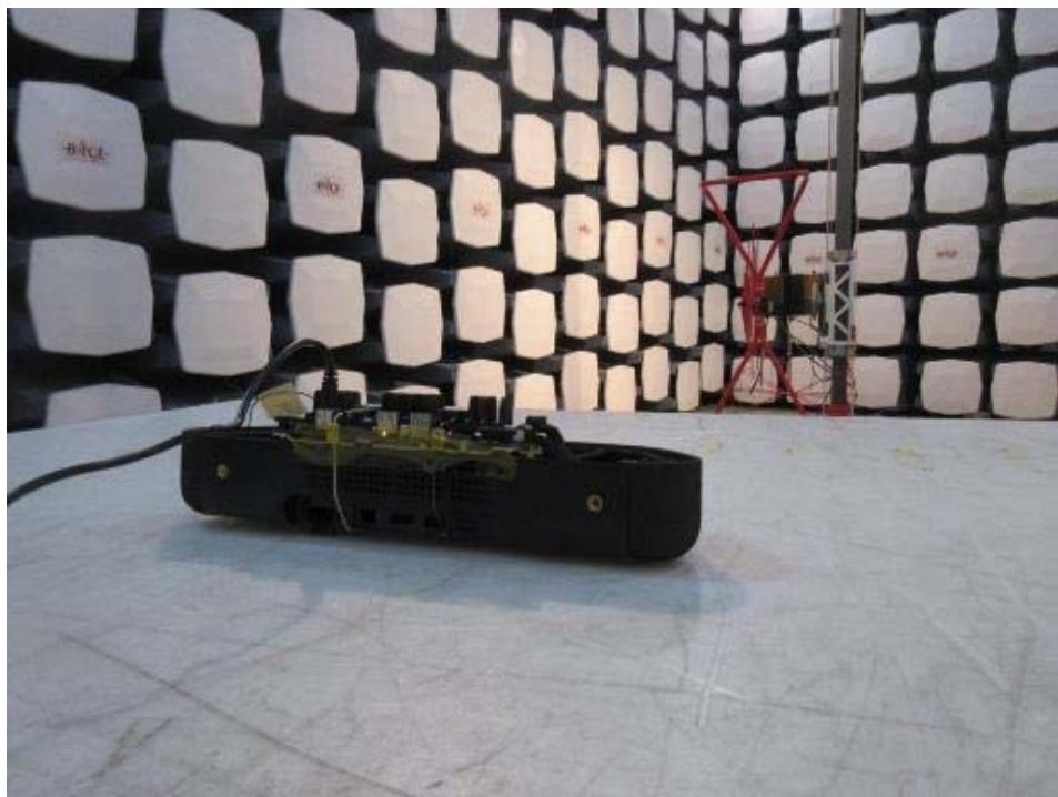
**1.3 Radiated Spurious Emissions: 1-18 GHz Front View at 3 meters**
