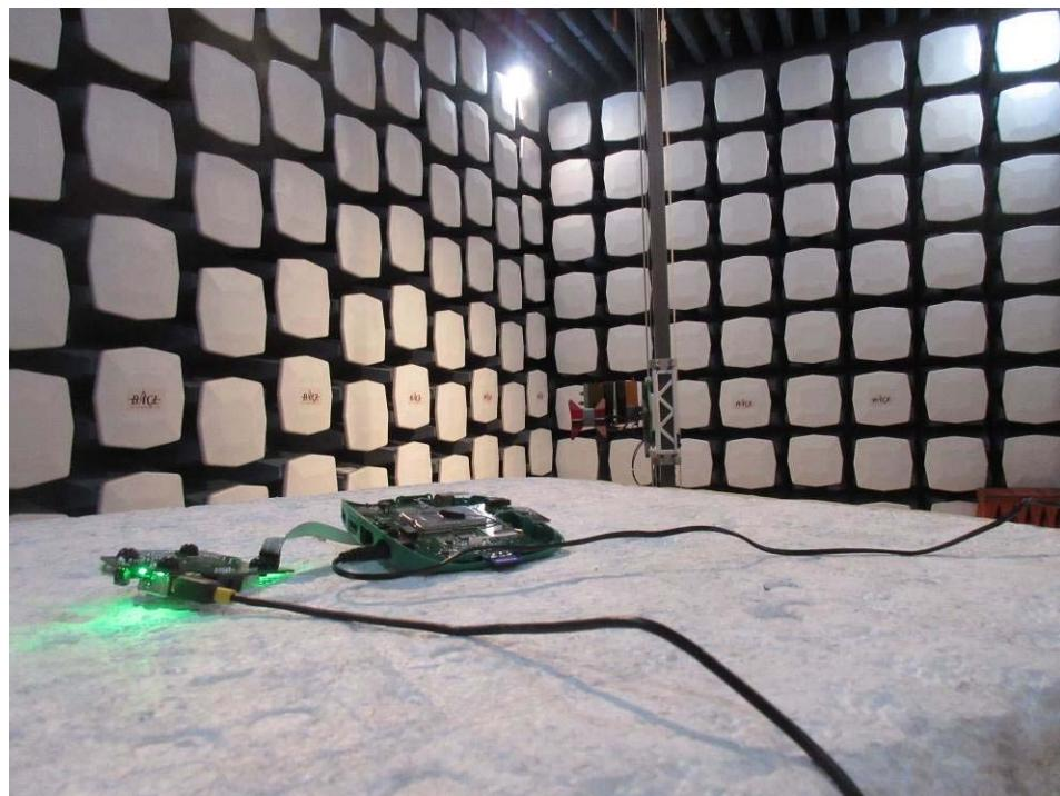
**1.5 Radiated Spurious Emissions: 1-18 GHz Front View at 1 meter**
