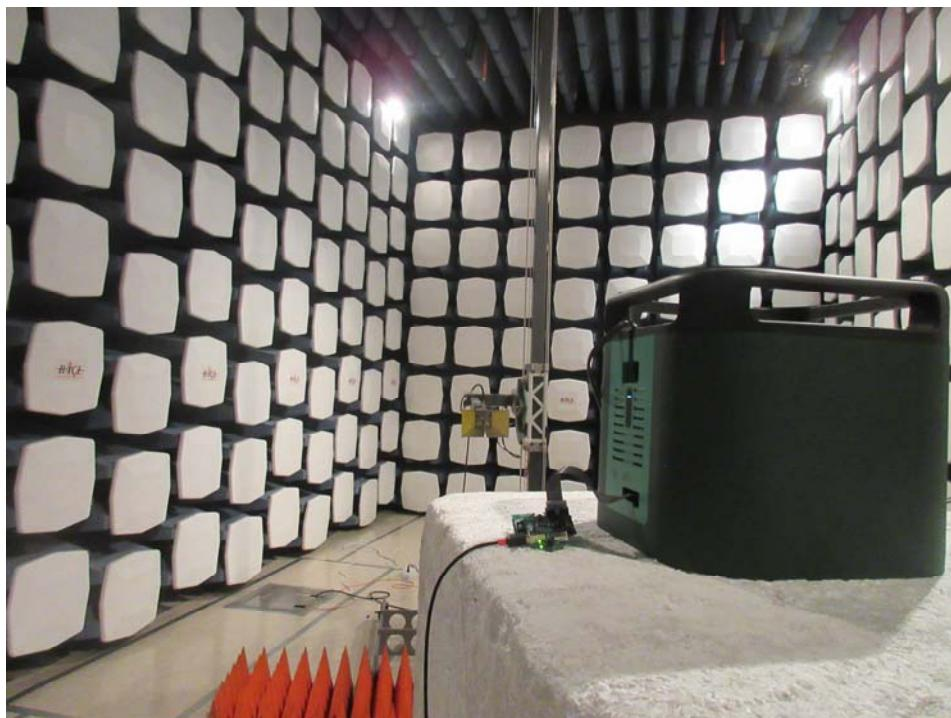
**1.5 Radiated Spurious Emission 1-18 GHz at 1 meter Front View**
