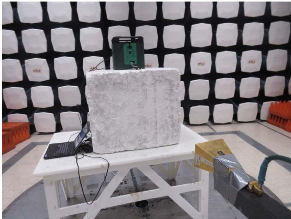
**1.8 Radiated Spurious Emission 18-26.5 GHz at 1 meter Rear View**
