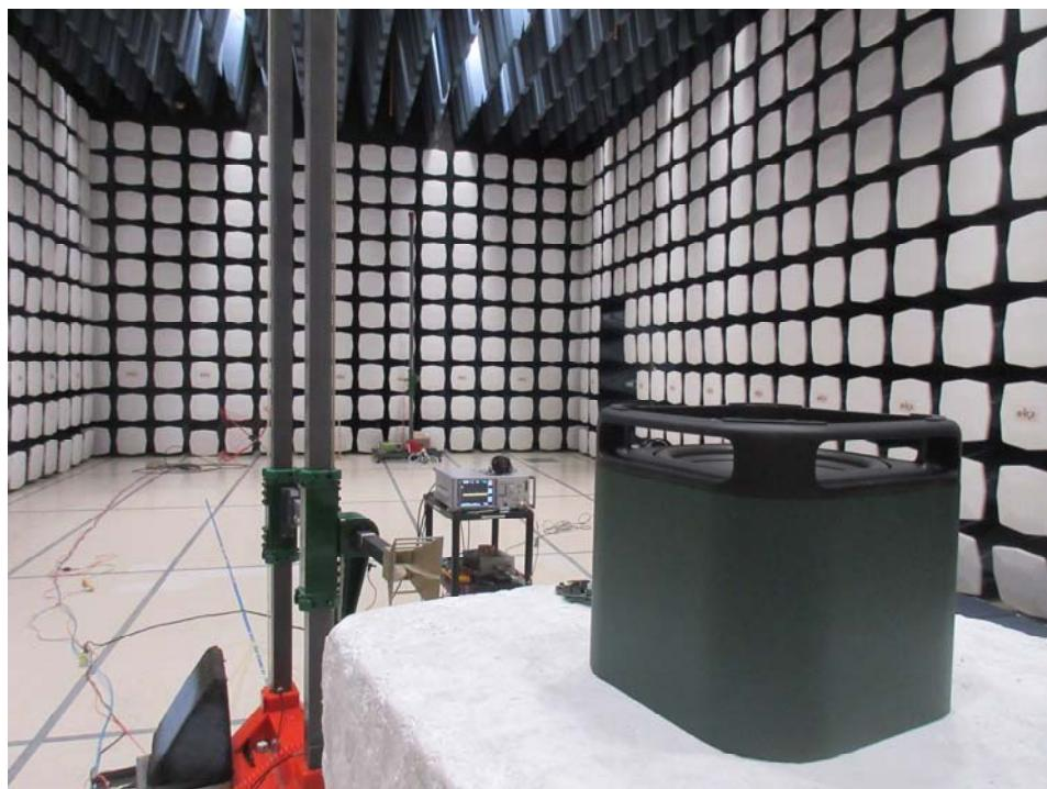
**1.7 Radiated Spurious Emission 18-26.5 GHz at 1 meter Front View**
