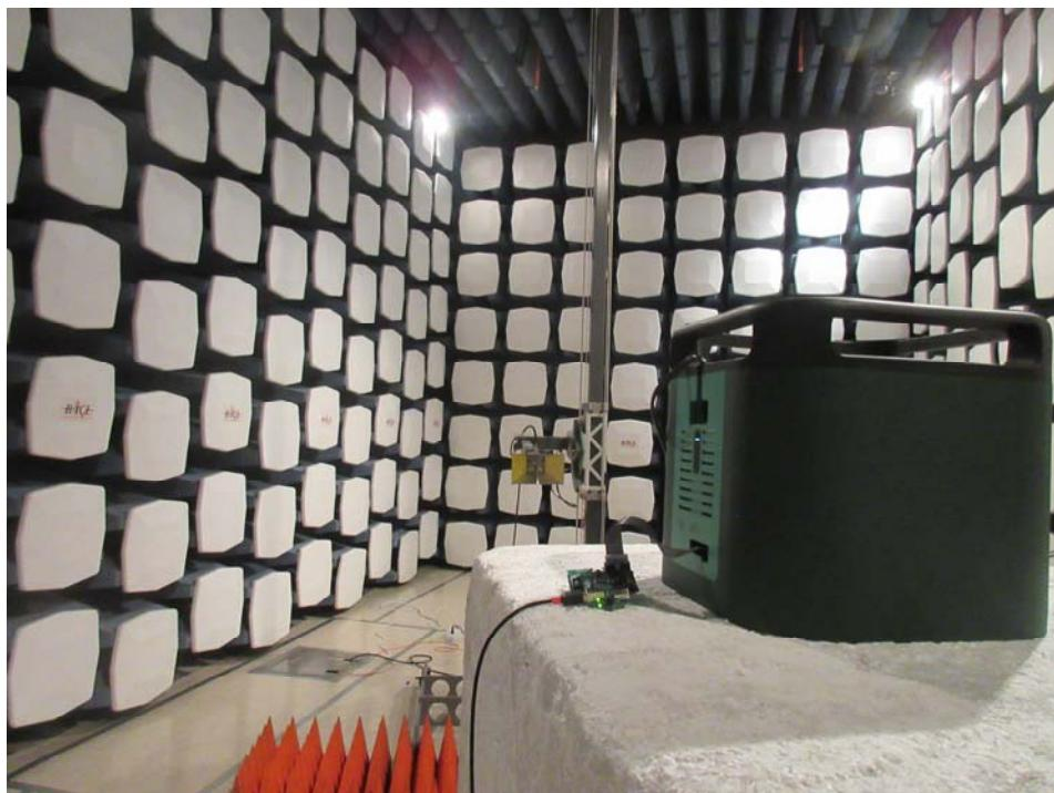
**1.5 Radiated Spurious Emission 1-18 GHz at 1 meter Front View**
