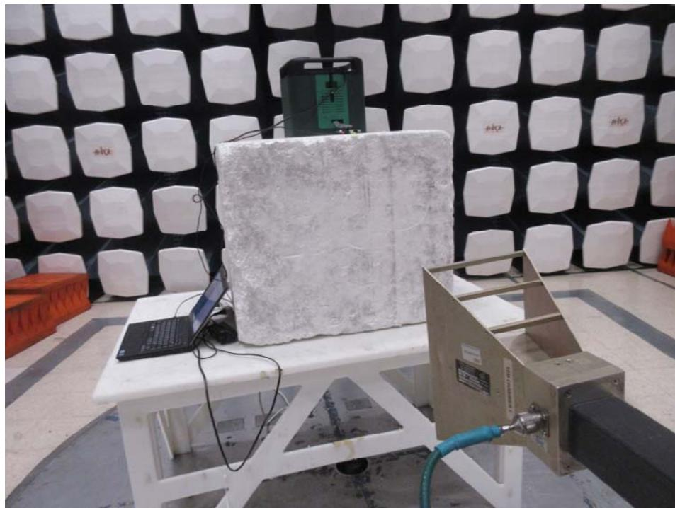
**1.6 Radiated Spurious Emission 1-18 GHz at 1 meter Rear View**
