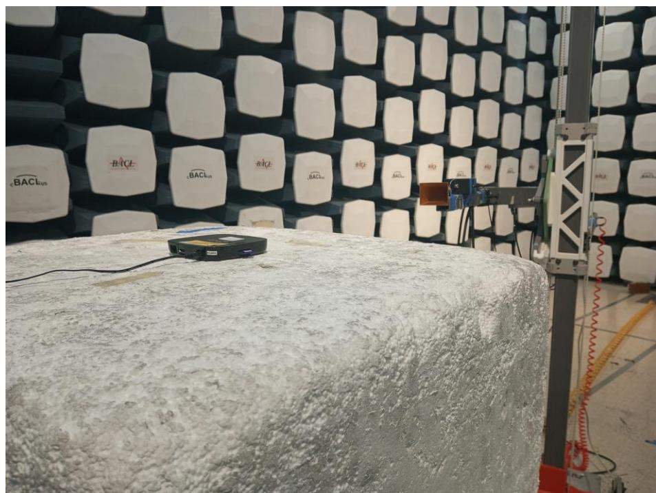
**1.7 Radiated Spurious Emissions: 26.5-40 GHz Front View at 1 meter**
