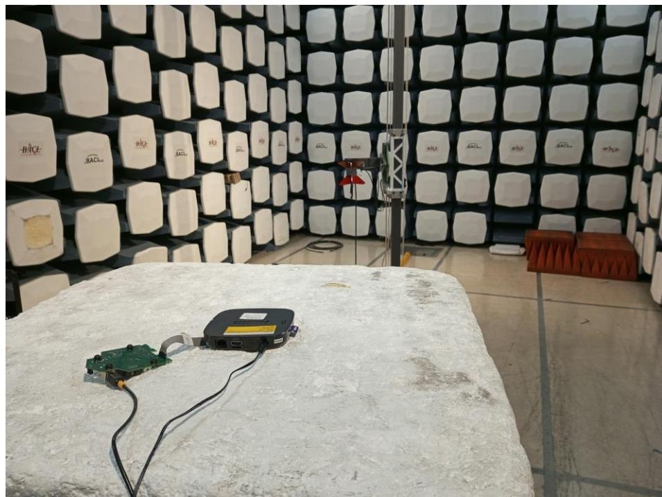
**1.5 Radiated Spurious Emissions: 1-18 GHz Front View at 1 meter**
