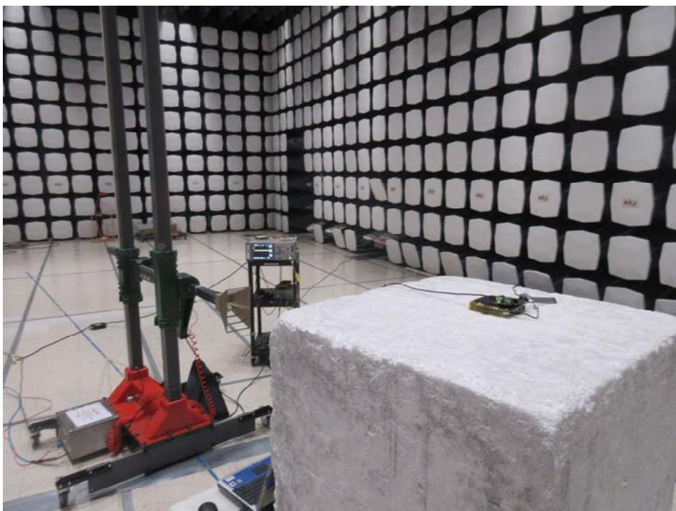
**1.5 Radiated Spurious Emission 18-26.5 GHz Front View**
