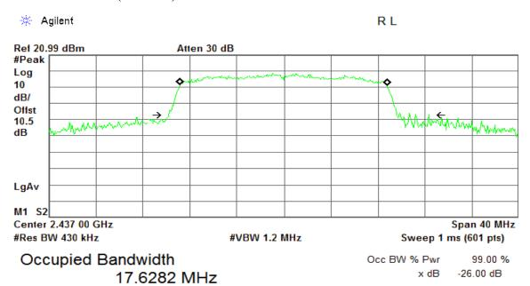
Transmit Freq Error -26.815 kHz x dB Bandwidth 22.126 MHz
