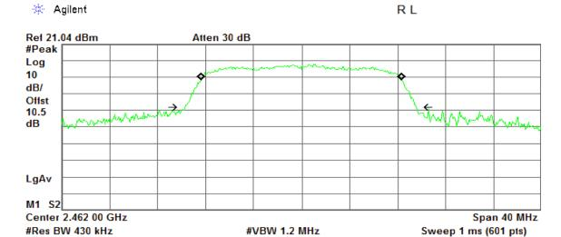
Occupied Bandwidth 16.7004 MHz Occ BW % Pwr 99.00 % x dB -26.00 dB
