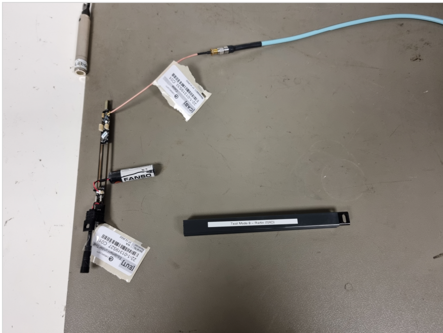
Photograph 7: EUT test setup for conducted measurement, close up view
