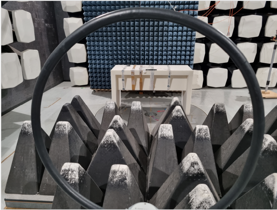
Photograph 1: EUT test setup in the semi anechoic chamber, measurement <30 MHz, overview
